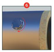
**STEP 6** Screw the metal cover onto the flange until tight and secure.
